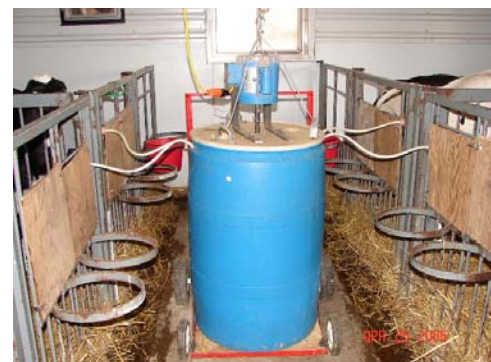
Figure 17. At a Milverton-area farm, a dose of old-fashioned ingenuity from a young farmer assures an even mix throughout the day. His storage and mixing system consists of a barrel, a 1/3-HP motor to drive a mixer and two timers to control frequency and duration of mixing. The motor mounts to a lid. A cart makes easy work of moving the barrel for washing and filling. Cables attach to the lid in three locations and they support the mixer above the barrel when moving the barrel away.
