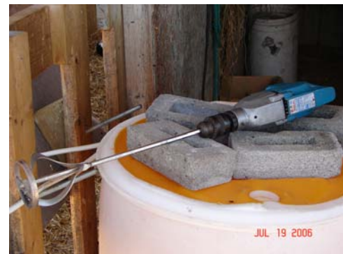
Figure 16. An electric drill and a paint stirrer attachment do a very good job of mixing. Several producers made mixers to insert into their electric drills. It is essential to select a mixer for the size of the container and volume of milk. For example, the smallest commercially available paint mixer is not adequate for mixing milk in 20-L pails or 100-L barrels.
